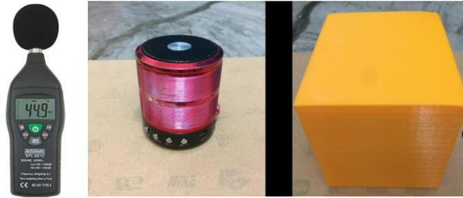
**Figure 1.6** Sound Reductions Experimental Setup consists of Sound Level Meter, Wireless Speaker, and Acoustic Enclose Sample
