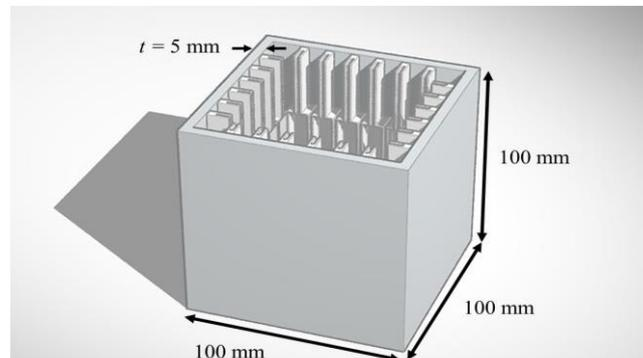
**Figure 1.2** 3D Acoustic Metamaterial Designed
