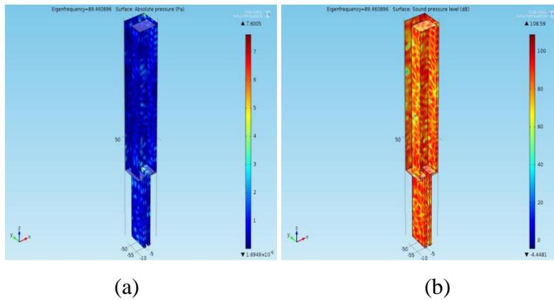
**Figure 1.7** AP on (a) Volume and (b) Surface of Unit Cell Geometry
