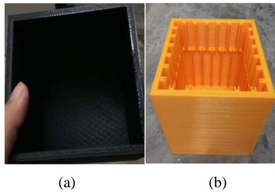
**Figure 1.5** 3D Printed of (a) Acoustic Enclosure and (b) Acoustic Enclosure with Metamaterial
