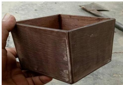
**Figure 1.3** Wood Acoustic Enclosure with Dimension of  $100 \text{ mm}^3$
