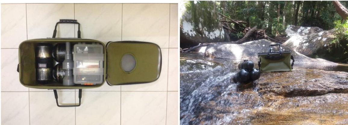
**Figure 1.0:** The Capsule Hydro Twin-Turbine (CaHT) and The CaHT on display
