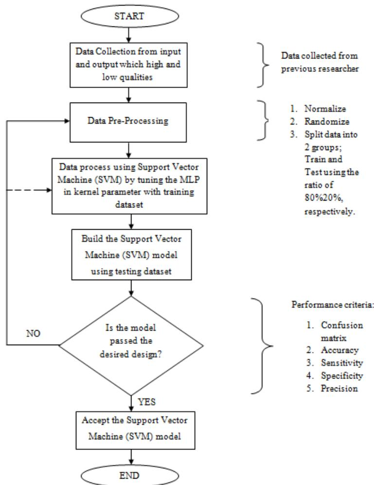
Figure 6 Flow Chart of Experiment Set-Up
