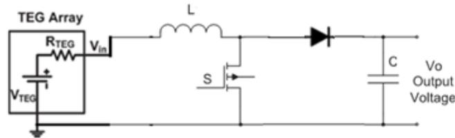
Figure 16. The schematic diagram of boost converter [21]
