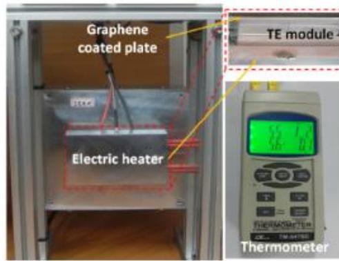
**Figure 15.** Application TEG at electric heater [17]
