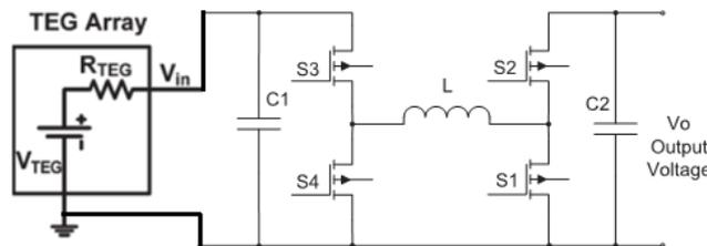
Figure 17. The schematic diagram of buck boost converter [22]
