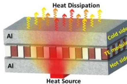
**Figure 13.** TEG system without graphene [17]
