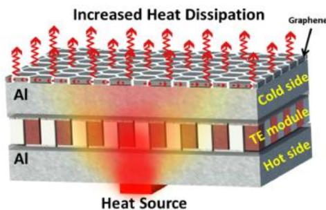
**Figure 14.** TEG system with graphene [17]
