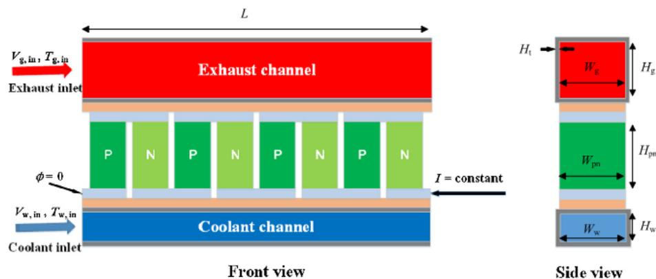
**Figure 5.** Energy harvesting from car exhaust [11]
