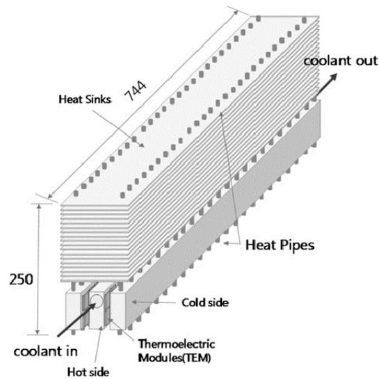
**Figure 10.** The prototype of TEG system for application at car radiator [15]
