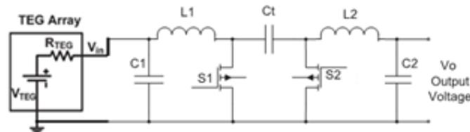
**Figure 19.** The schematic diagram of CUK converter [24]
