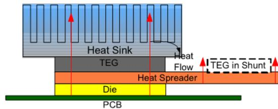
**Figure 8.** The schematic diagram of TEG system [14]
