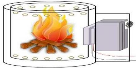
**Figure 12.** The schematic diagram for application TEG at cook stove [16]
