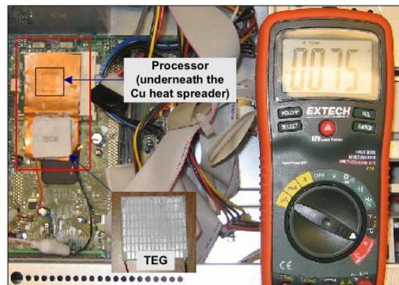
**Figure 9.** The system setup of TEG system [14]
