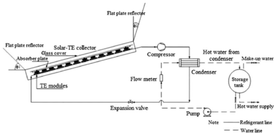
**Figure 6.** The schematic diagram of the TEG system for application at roof top [12]
