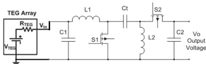
Figure 18. The schematic diagram of sepic converter [23]
