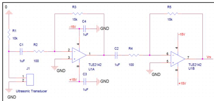
**Figure 2.2** Signal Conditioning Circuit
