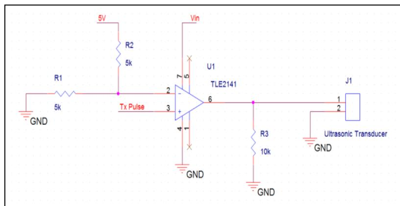
**Figure 2.1** Pulse Generator Circuit schematic
