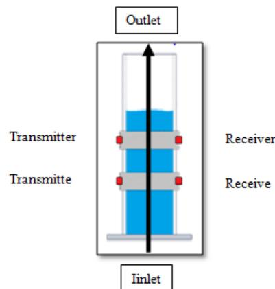
**Figure 1.1** Sensing area consists of 2-pairs of ultrasonic transducers.
